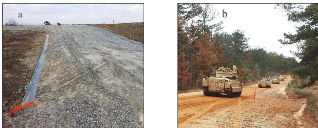
Figure 3. In the Fort Benning road erosion study: (a) Grab sample plot on the improved site. Note the natural slope break serving as the top of the plot, the metal side gutter, the shallow trench diverting water from the bottom of the plot to the collection point, and the gray color of the compacted aggregate; and (b) military vehicles on the unimproved plot. Note the deposition in the road ditch leading to the inlet to the collection pipe (fig. 5), the rills delivering sediment to the ditch, the ruts forming on the road from the traffic, and the red hue of the weathered loamy sand soil.
